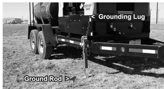
Figure A8 Set and Connected Ground Rod
