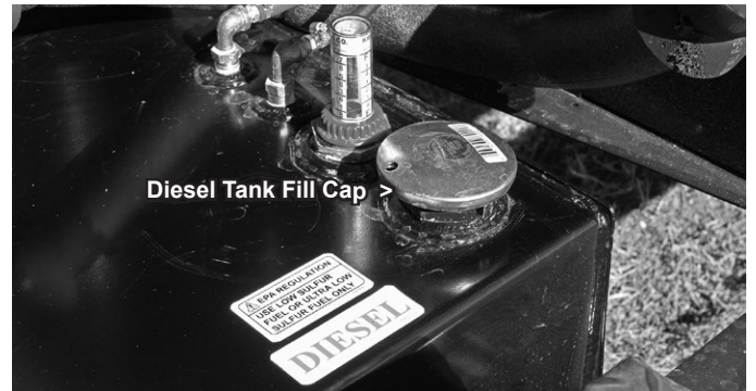
Figure A7 Diesel Tank Fill Cap Setting the Ground Rod
