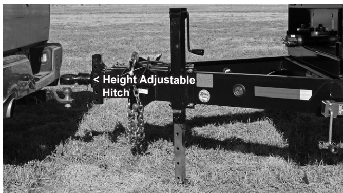
Figure A5 Adjust Hitch Height for Level Trailer
