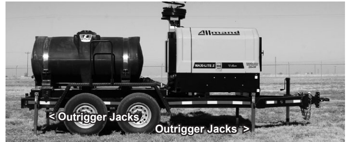
Figure A6 Set Outrigger Jacks to Stabilize Trailer
