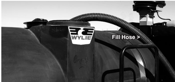
Figure B1 Filling Tank Through Fillwell
