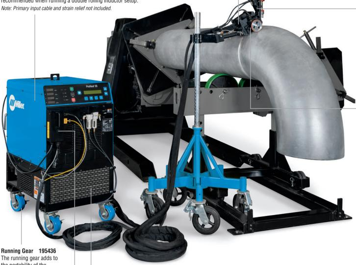
The running gear adds to the portability of the system. The four 5-inch swivel casters with brakes mount to the bottom of the
