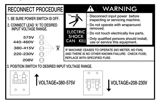
Figure A.1 Input Voltage Reconnect Instructions
