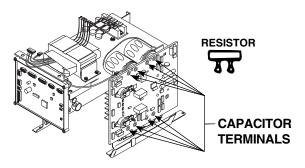
3. Use a DC voltmeter to check that voltage is not present across the terminals on all four capacitors.
