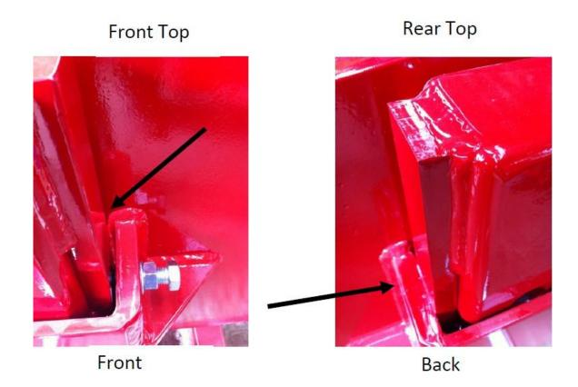
Note the vertical leg (with holes C through), is designed to sit flush, metal on metal at the top rear and bottom front of the sleeve (see pictures above). These areas are designed to take the weight of the machine. The bolts (D) are there to close the gap at the top front and bottom rear of the sleeve, so that there is no movement of the position in the sleeve.
