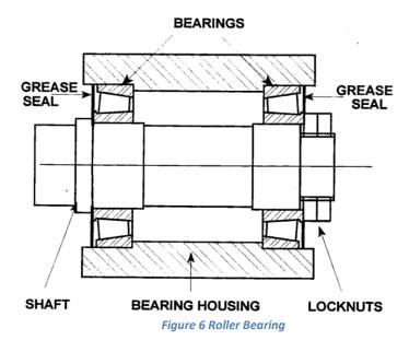
Replenish at 500 hour intervals with CASTROL SPHEEROL MP3. For high temperature conditions change grease to CASTROL SPHEEROL B3.
