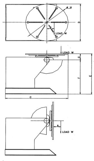
ROTATION TORQUE (R) IS A STRAIGHT FORWARD CALCULATION OF LOAD (W) X ECCENTRICITY (B) BUT TO ENSURE AN ACCURATE FIGURE FOR TILT TORQUE (T) IT IS IMPORTANT TO USE THE FULL DISTANCE TO THE PIVOT POINT. THIS IS OBTAINED BY ADDING TOGETHER THE CENTRE OF GRAVITY (A) AND TABLE PIVOT DISTANCE (G). THEREFORE :-ROTATION TORQUE (R) = W X B Kg METRES TILT TORQUE (T) = W X (A + G) Kg METRES MULTIPLY BY 9.81.
