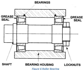
Replenish at 500 hour intervals with CASTROL SPHEEROL MP3. For high temperature conditions change grease to CASTROL SPHEEROL B3.
