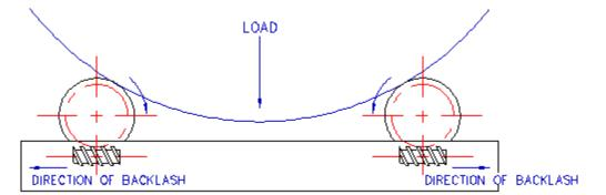
FIGURE 8 - BACKLASH ALWAYS LOADS OPPOSITELY AS THE VESSEL CRADLES INTO WHEELS
