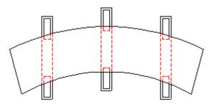
FIG. 11D - MISALIGNMENT, PLAN VIEW
