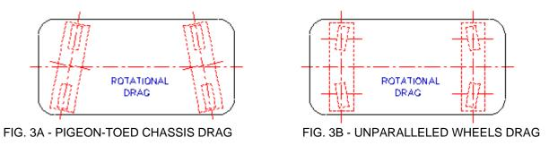
A solution to some misalignment problems may be obtained by placing a smooth, flat steel plate on a leveled section of shop floor and letting the rolls rest on the plate without them being lagged down. This allows the
