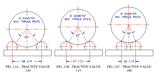
As shown in Figures 11A, B and C, a turning roll with adjustable center-distances will accommodate a given diameter vessel in more than one Center-Distance setting. For example, a PRESTON-EASTIN turning roll will cradle a 6-foot vessel in C-D settings of 36.25", 47.5" and 58.75". USE A SHORT CENTER DISTANCE WHENEVER POSSIBLE. Symmetrical, balanced vessels will safely cradle in contact angles between 45° and 60°.
