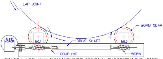
FIGURE 9 - NORMALLY, ONLY ONE WHEEL DRIVES WHEN ROTATING THE VESSEL
