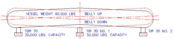
FIGURE 4 - INHERENT OVERLOAD: LONG VESSEL, BENT CENTERLINE, THREE ROLL UNITS
