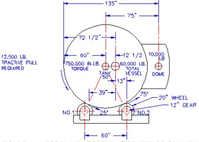
FIGURE 10 - VESSEL WITH ECCENTRIC CENTER-OF-GRAVITY
