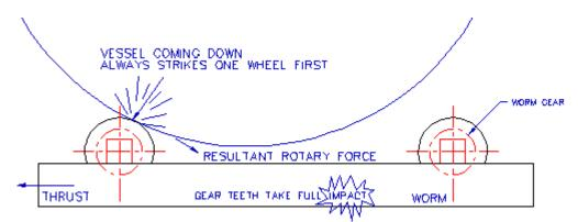
FIGURE 7 - WHEN LOADING THE VESSEL, IT ALWAYS STRIKES ONE WHEEL FIRST
